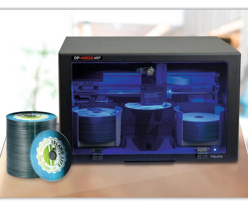
**DP-4202 XRP** automates the process of burning and printing quantities of recordable CDs, DVDs and Blu-ray Discs. Using built-in robotics, discs are transported one at a time into either single or dual optical drives. After data is burned, the discs are transported to a high-speed, high-resolution full-colour disc printer.
